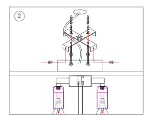
Connect the power cord, fix the ceiling plate on the hanging board with screws on the side / install the light source and try to light it
