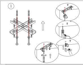
Take out the cross hanging plate, and fix the cross hanging plate on the outlet position of the ceiling (it is recommended to use tapping expansion screws)
