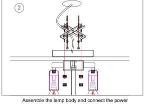
Assemble the lamp body and connect the power cord, fix the ceiling plate on the hanging board with sprig nuts/install the light source and try to light it (if hoisting is required, remove the ceiling plate and add a hanging chain in the middle)
